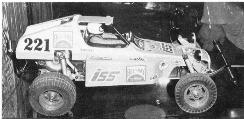
Tamiya's off-road car hydraulic springing to all four wheels and thoroughly stout construction all round.
